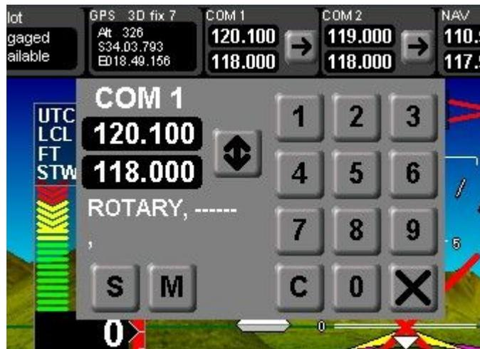
Here we have tapped on the COM 1 radio to bring up a larger version. Depending on the type of radio connected we can interact with the radio at various levels. Just flipping frequencies however requires only a tap on the displayed frequencies on the small COM 1 display (with animation so it is easy to see what is happening). If a MGL radio is connected, the radio can be fully remote controlled from here – including volume, squelch and even all of the radios setups.
