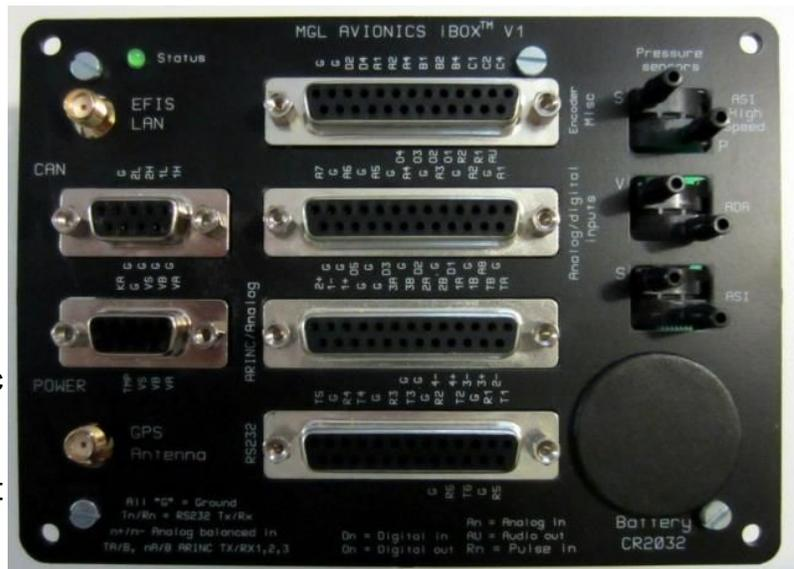
Each iBOX provides a low speed (16-250mph) airspeed sensor and an optional high speed sensor capable of several mach numbers at altitude. Both sensors are used so even if a high speed sensor is specified, no resolution is lost at low speed. Altimeter with a 1 ft resolution to above 40.000ft is standard as is a built in AOA sensor that can be used for both differential as well as single ended measurements.
