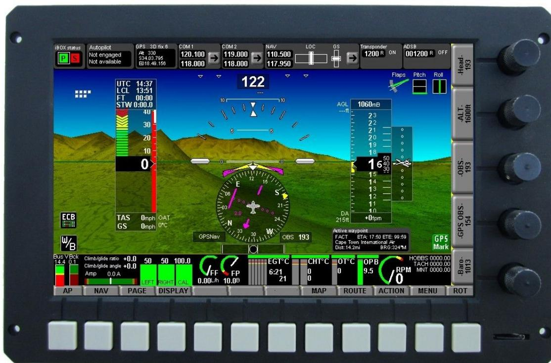
The Explorer EFIS introduces a custom developed touch pressure sensitive LCD screen aimed exclusively at the small aircraft application. With the ability to accurately measure contact force in all conditions, it becomes possible to utilize the user interface advantages of a touch screen even in turbulent flight.
