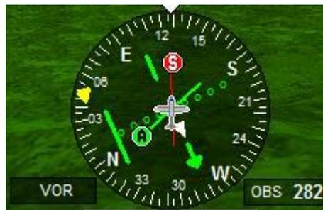
VOR NAV is described in more detail further down in this document. The system provides for a primary and secondary VOR source showing “paddles” that give you an indication where these sources are located (from a direction point of view). The radials from these VOR stations are shown as lines.
