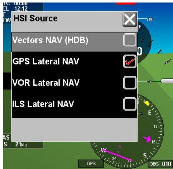
Selecting a GPS waypoint, activating a route (flightplan), selecting GVOR primary or activating a GLS selects the navigation source automatically.
