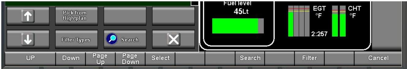
Note that most touch screen functions are also duplicated by means of the soft key buttons below the screen (except on iEFIS Lite systems).
