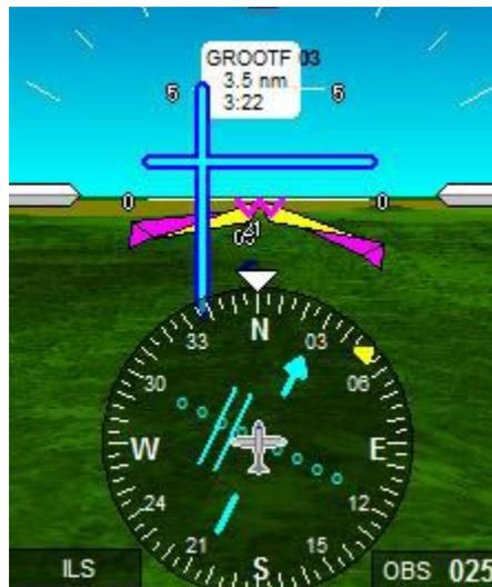
Textual information shows that we are 3.5 nm from GROOTF and need 3 minutes, 22 seconds to touch down at current speed. The HSI shows we are to the right of the runway. This is confirmed by the light blue ILS needles in the screen center which show the glide slope above us to our left.
