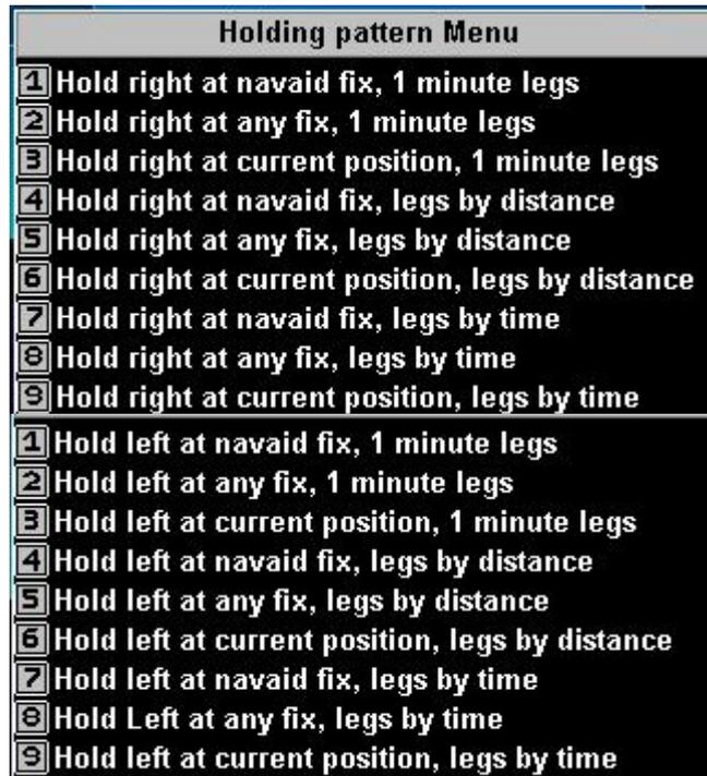
Holding patterns can be located at a navaid (such as a VOR), any fix (Waypoints etc) or at the current position.
