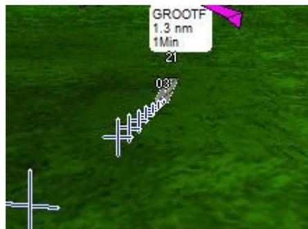
This image shows approach guidance onto runway 03 at GROOTF. Approach guidance is shown with blue crosses on a white background. The glide slope angle is based on the angle selected in your GLS setup (typically 3.0 degrees).
