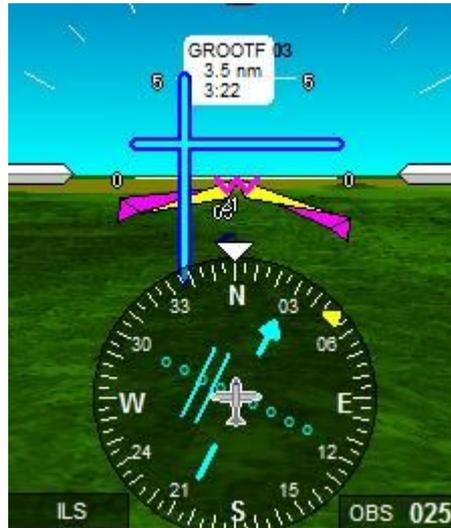
Textual information shows that we are 3.5 nm from GROOTF and need 3 minutes, 22 seconds to touch down at current speed. The HSI shows we are to the right of the runway. This is confirmed by the light blue ILS needles in the screen center which show the glide slope above us to our left.
