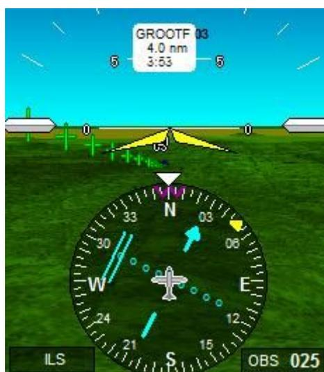
The GLS approach uses white crosses on a green background to distinguish from the similar approach guidance. GLS, like ILS is a navigation source and can be used as source for the HSI and thus, the autopilot if engaged.
