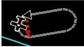
Image showing an active holding pattern on the moving map. With the holding pattern active, map background (terrain and cultural data) is suppressed.
