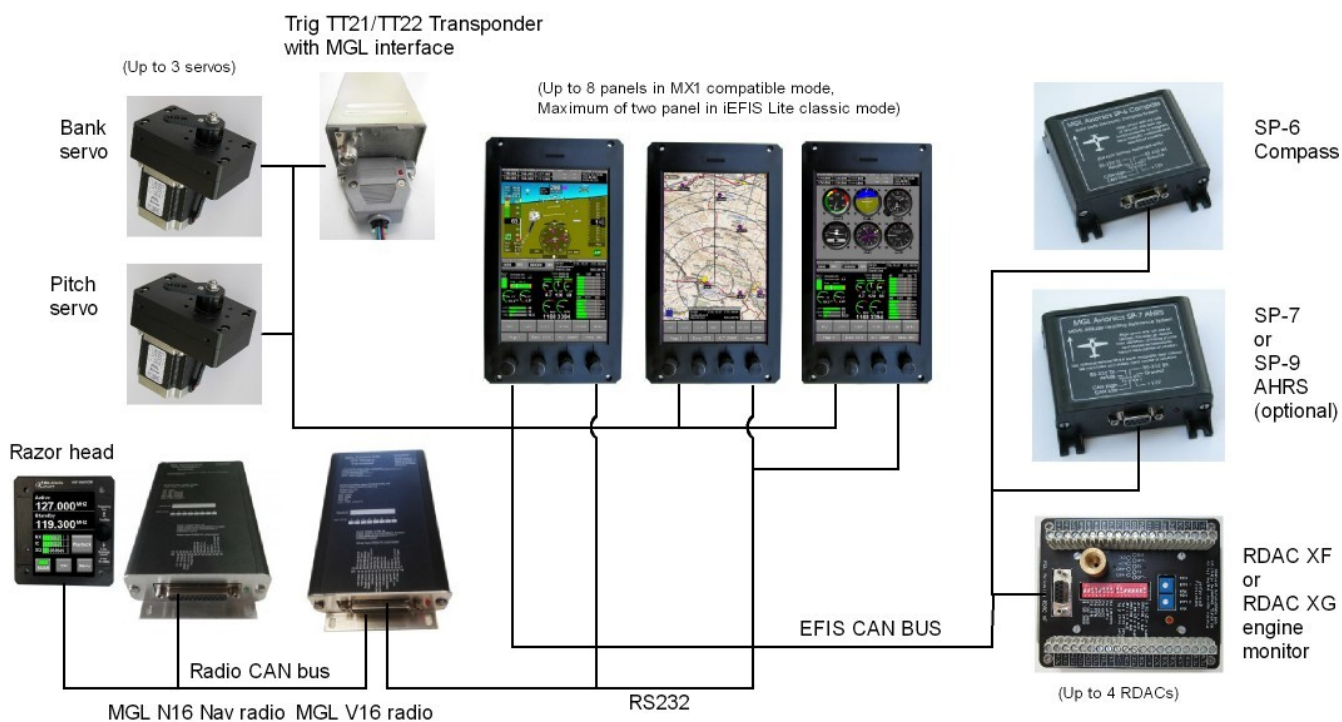
Example iEFIS G4 MX2 Lite system layout for a three panel solution, showing main communications bus connections.
