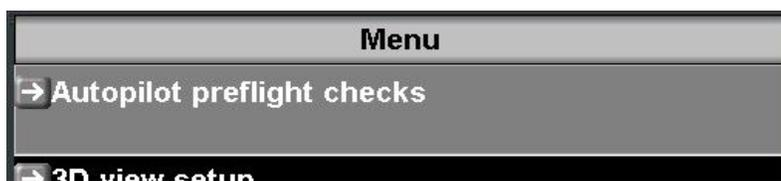
While the preflight check is operating, physically move the control surfaces by hand against the servo force to locate any play. If you find significant play, please fix the cause before attempting a test flight. The autopilot cannot perform correctly if there is excessive play in the controls.
