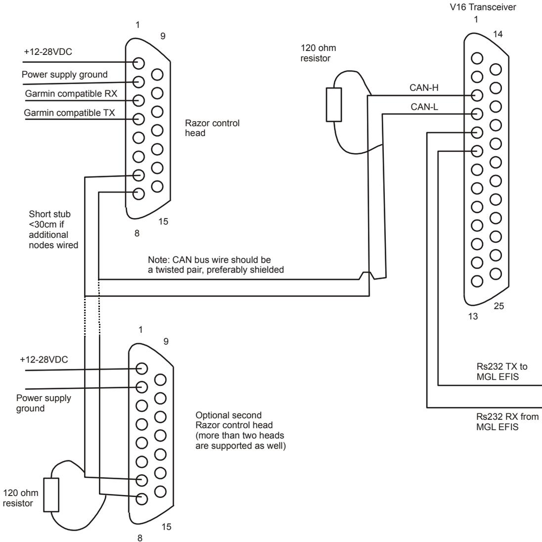
The V16 transceiver module must be connected to at least one controller. It is possible to operate the V16 without a control head if one has been used to setup volume and other settings. In this case only a single frequency is used (setup by the control head). All settings are stored in the V16 and maintained. This is an option for fixed base station use only.
