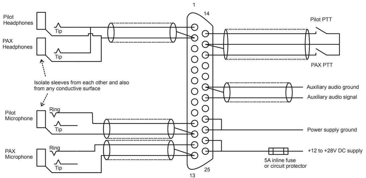
This diagram shows a typical two place setup for a pilot and single passenger for two
