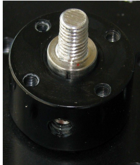
Output Shaft and Collar with Output Arm removed exposing 4 sets of thread for the Sheer Screw
