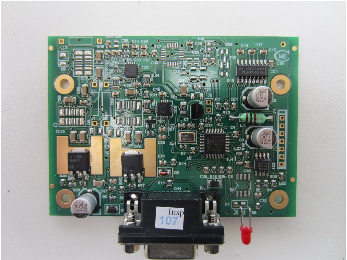
Picture of a current generation SP-7. **Do NOT** remove the capacitors.
