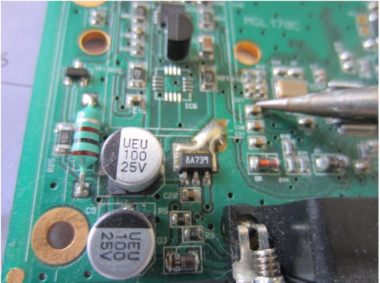
Apply heat to the capacitor until the solder melts and you can remove it. Here we are removing the first one (top of three).
