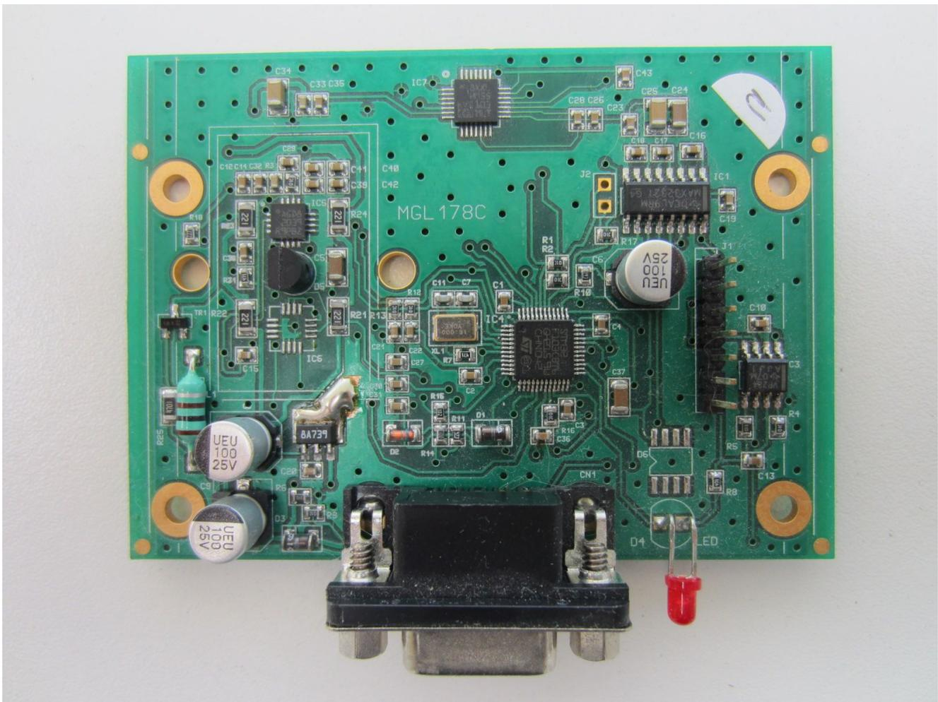
View of a first generation SP-7 PCB that needs to have the capacitors removed. They are labeled C30,C31 and C27.
