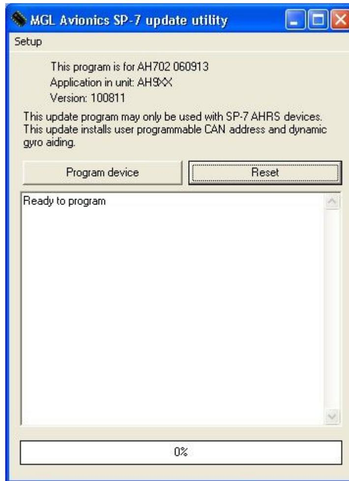
The version of firmware in your unit will be shown (Here it is 100811 which means August, 10<sup>th</sup>, 2011). We are about to program 060913.
