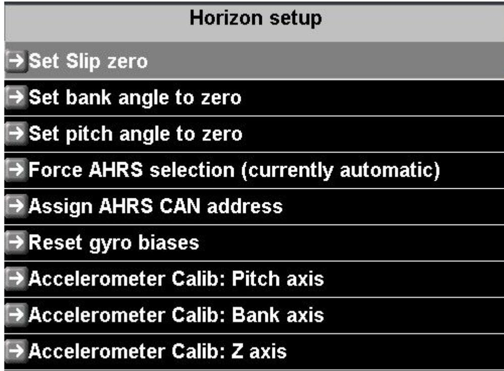
“Set Slip Zero”, “Set bank angle to zero” and “Set pitch angle to zero” are unchanged from previous releases. These functions are intended to be used to “fix” slight installation misalignment of the SP-7. Any corrections are stored in the EFIS, the actual SP-7 is not affected.
