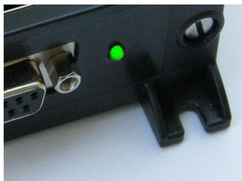
The green LED flashes at about 1Hz during operation. If the LED is steady "ON" there is a serious fault with the RDAC and it cannot operate. If the LED is "OFF" the RDAC is not being supplied with power or there is a serious fault with the RDAC. If the RDAC is connected to an EFIS the LED will perform a double flash to indicate that it is "seeing" the EFIS.
