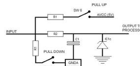
These circuits shows how the various PU switches feeds 5 volt onto the input(sense) line if required. Please check the senders information for type and settings needed. The 2<sup>nd</sup> circuit shows a pull down circuit that has a 100Ω load resistor switched to GND. This intended for use with the Rotax 4-20 mA oil pressure sender. The white wire is connected to the OILP input on the RDAC XF. The OILP PD switch must be in the ON
