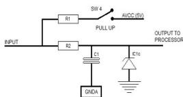
This drawing illustrates the pull up and pull down resistor circuit for the oil pressure
