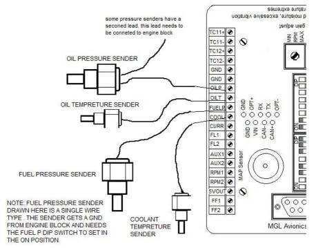
It is important to know what type, range and connections are needed for the sensors. In the EFIS and I-EFIS units menu's relating to the sensors placement can show you what sensor types can be used.
