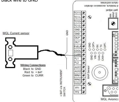
The magnetic current sensor can be installed in several ways depending on the current range it is to measure. Please refer to the documentation for this sensor.
