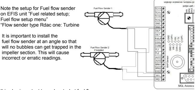
It is also important to work out what fuel flow to expect (generally manufacturers specify fuel usage per hour) in order to select the right jet for the fuel flow sender unit.
