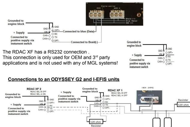
When using CAN interface, you can connect up to four RDAC XF s togetherer.
