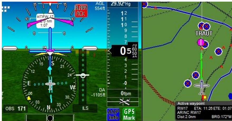
The new waypoint name will appear on the EFIS but the waypoint location can only be seen on the Garmin display. In the example to the left the pilot has selected VLOC on the GARMIN “CDI” Key, and has switched the NAV receiver to the KCEW ILS localizer frequency, and finally
