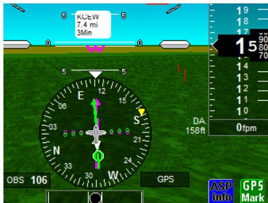
Garmin VLOC frequency Key which moves the CEW VOR frequency from the standby to the active NAV frequency. The pilot should then see the EFIS HSI display go active when the Garmin receives a valid VOR signal, the
