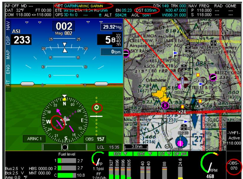
If BIT test is still not correct check the other EFIS and/or GARMIN interface settings. If there is no indication of ARINC communications between the two units then check the EFIS ARINC Bus Analyzer (shown below). If BIT test is successful then press the GARMIN “ENTER” key and resume normal operations.
