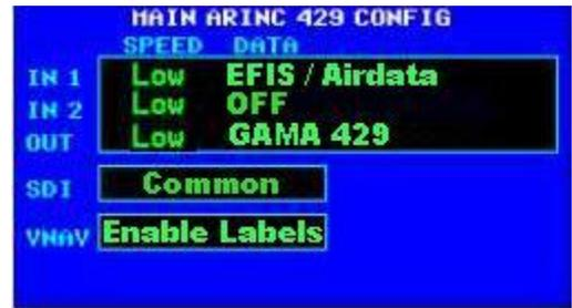
VNAV → Enable Labels (Allows GPS Vertical NAV)
