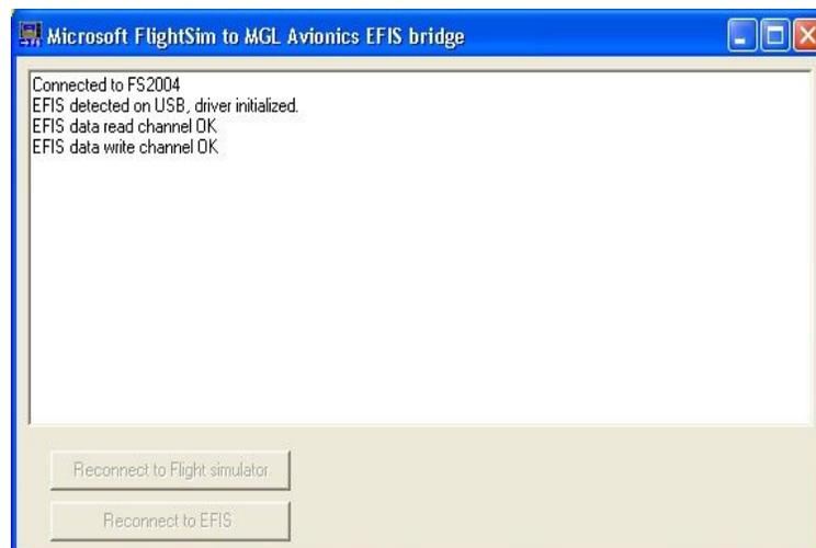
If you see the above window your EFIS is connected to your Flight simulator. Primary flight instruments, AHRS and GPS related items should now be functional.
