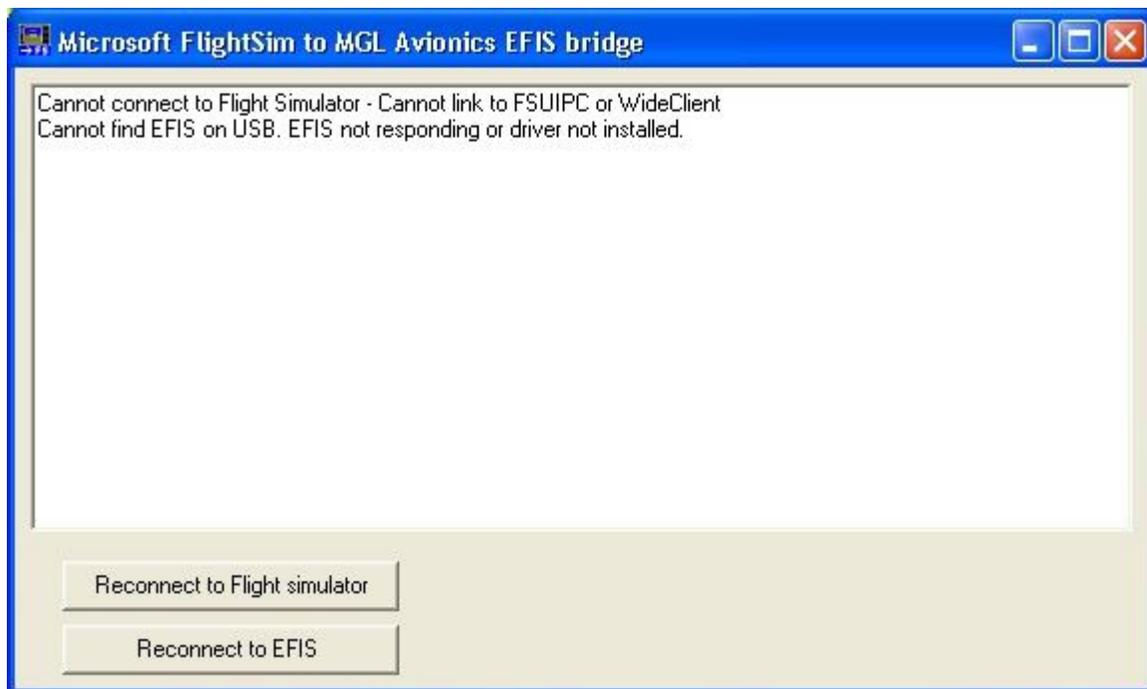
This is the window of the MGLUEFIS program. In this case it has not been able to connect to either Microsoft's Flight Simulator or an MGL EFIS. This is expected for a new installation as you will need to do some more work...
