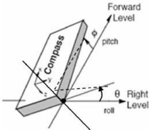
This graphics illustrates the problem. The X and Y sensor readings of the compass are used to calculate the heading. This is trivial but only gives you the heading you want if the compass is perfectly level to the Earths surface.
